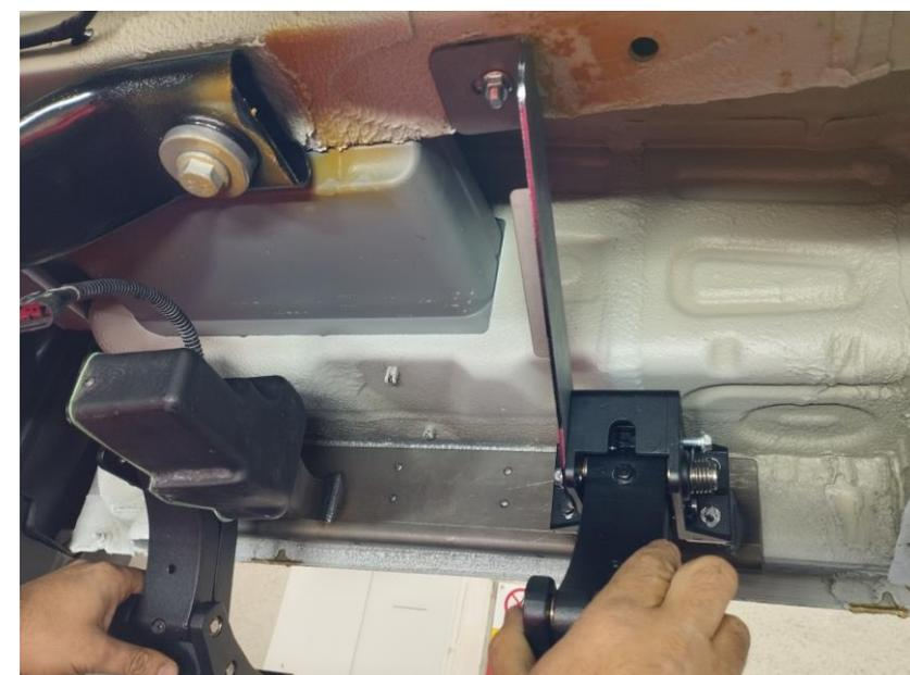
Installation of the rear connecting bolt of the carrier chassis on the vehicle is made as shown in the picture.
